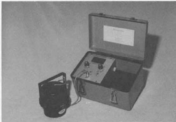
Acoustic well sounders use sound waves to measure depth. (Photo courtesy of Toole & Sons Drilling. Used by permission.)
